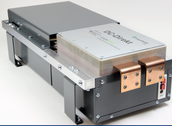
Side view of full bridge cell with power busbars and fiber-optic cable connectors
